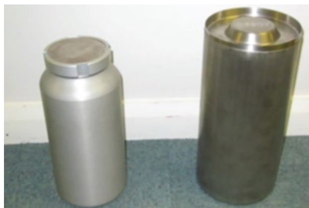
Figure 1: A photograph of the inner container of a Magnox package on the left, and the outer container on the right. (2)
