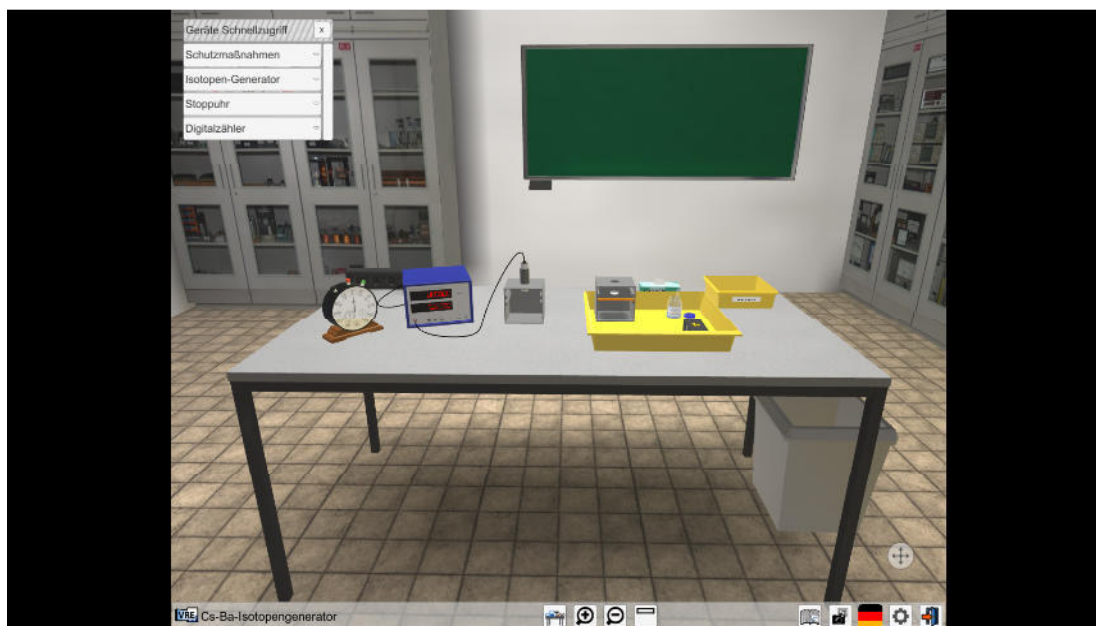
Fig. 1 general set-up of the VRE to determine the half-life of Ba-137m
