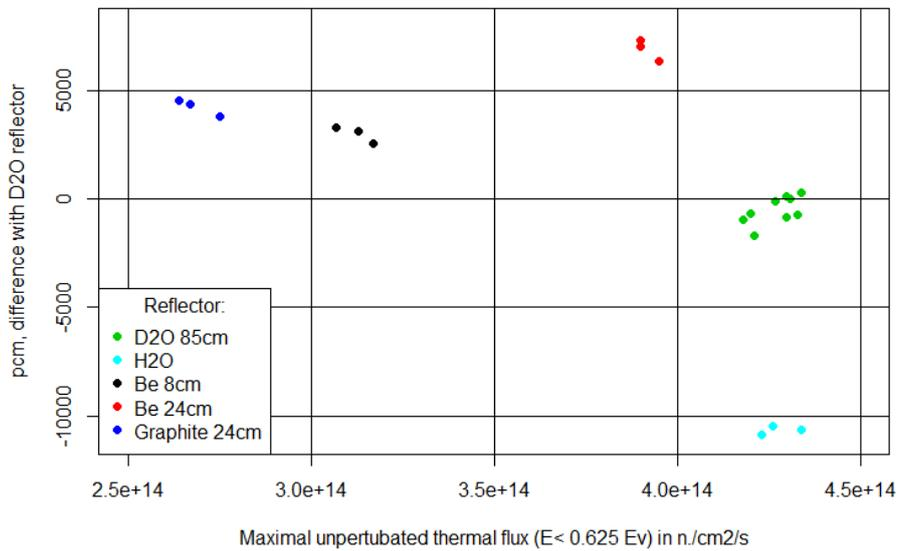
Figure 6: Core reactivity - Comparison between pure D<sub>2</sub>O, H<sub>2</sub>O, fresh Be-block with water gaps and graphite
