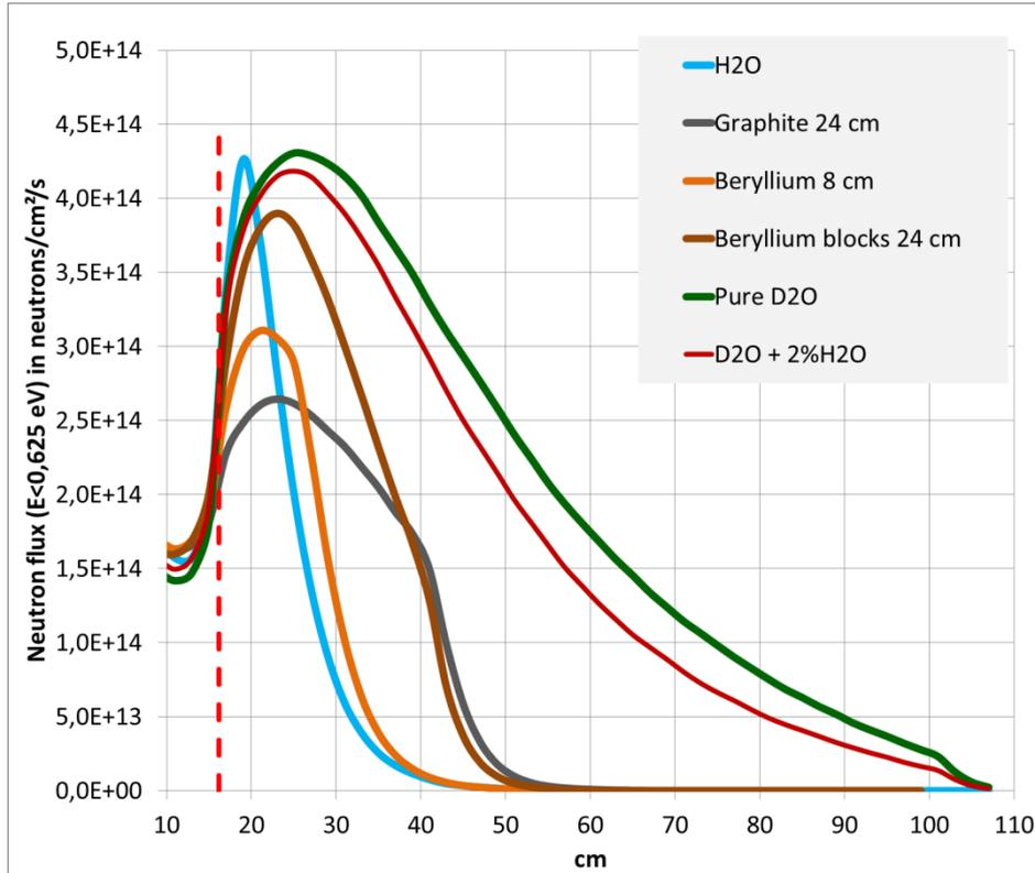
Figure 5: Thermal neutron flux reactivity - Comparison between pure D<sub>2</sub>O, H<sub>2</sub>O, fresh Be-block with water gaps and graphite
