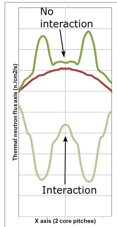
Figure 1: Example of potential interaction between 2 in-reflector devices.
