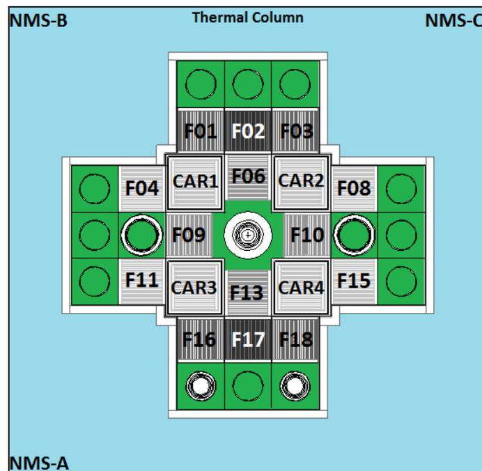
Fig 1. JRTR Core Configuration
