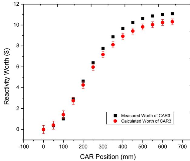
Fig 3. Measured and calculated worth for CAR3
