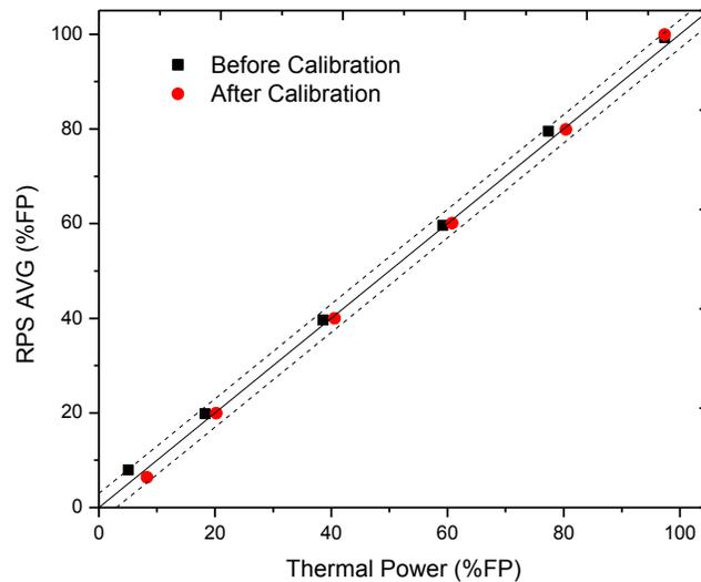
Fig 4. Power readings of the thermal and the RPS signals, before and after (re)calibration.
