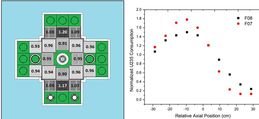
Fig 2. Normalized U<sup>235</sup> Consumption Distributions
