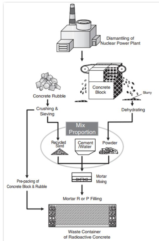
Fig.6. Method of radioactive concrete utilization for mortar [6]
