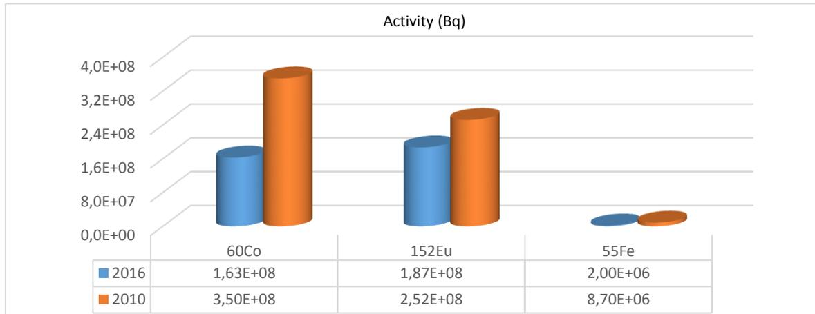
Fig.3. Radionuclide inventory for concrete biological protection
