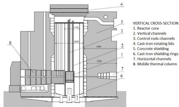
Fig.2. Vertical cross-section of the reactor block
