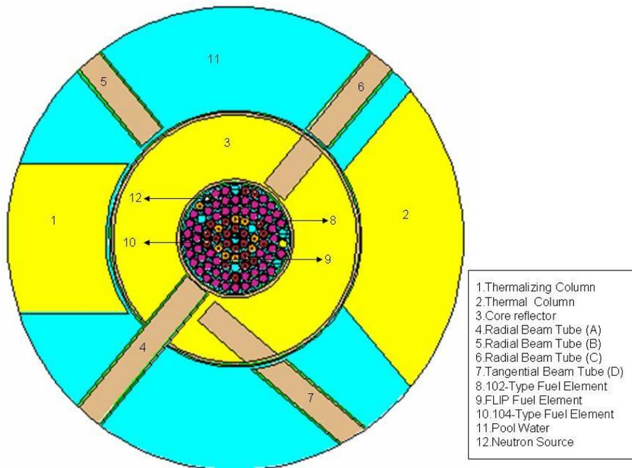
Figure 2: Horizontal cross section of the TRIGA Mark II core in Vienna 2008
