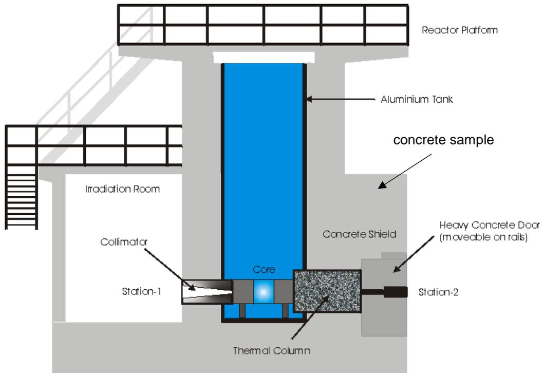
Figure 1: vertical view of the reactor with concrete sample position
