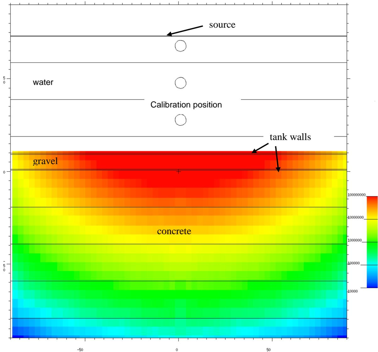
Figure 3: neutron flux below at the reactor tank bottom
