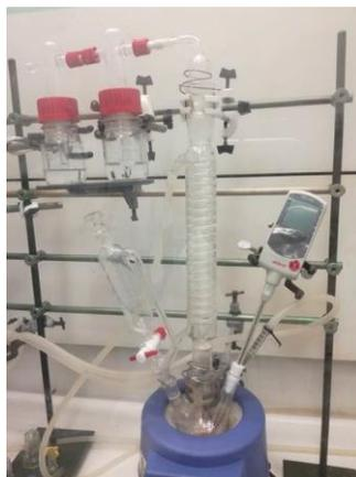
**Figure 7: Setup for the IER destruction**
