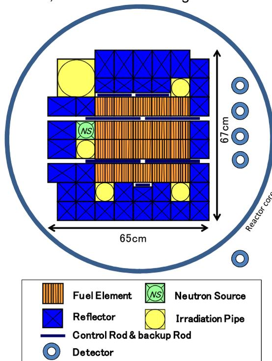
Fig 3. Layout of the reactor core of JRR-4
