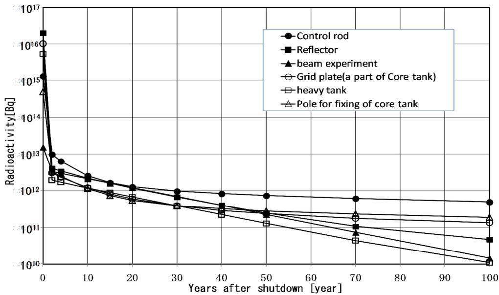
Fig.6. Change of activation radioactivity of main structures
