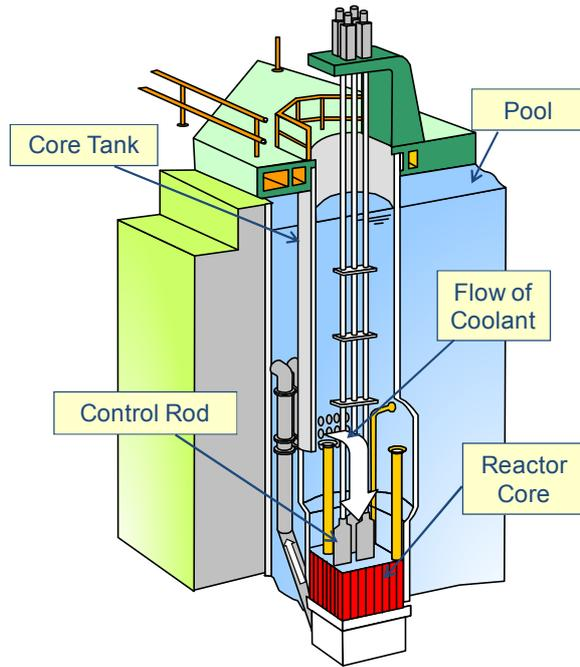
Fig 2. Cutaway view of the core tank of JRR-4
