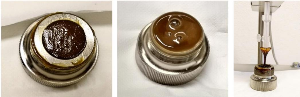
Figure 4. Grizzlygrease No.1 irradiated at 0.14 MGy (left) and 0.42 MGy (center). The grease became almost fluid after irradiation (centre). Klüberlub BE 41-542 grease irradiated at 4.39 MGy, becoming almost fluid (right). The grease drips from the instrument. Consistency is measured using a penetrometer.
