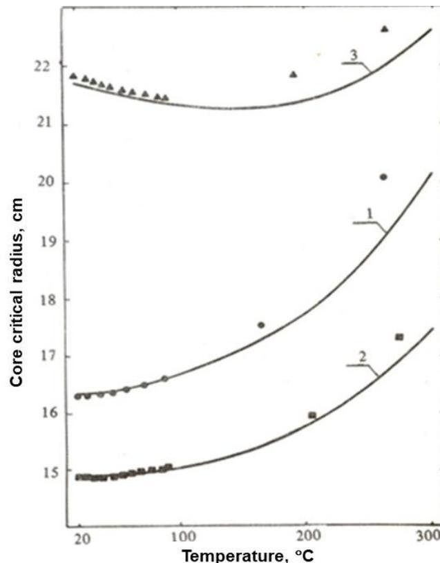
Fig. 2. Critical radius of hexagonal fuel rod bundles depending on temperature:
