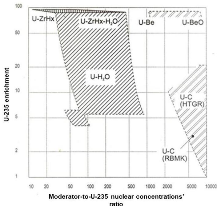
Fig. 1.  $^{235}\text{U}$  enrichment and moderator-to- $^{235}\text{U}$  uranium nuclear concentrations' ratio in critical experiments performed in the Kurchatov Institute
