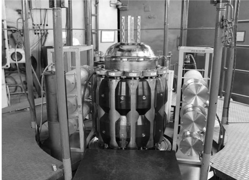
Fig. 3. Critical assembly simulating RP-50 thermionic converter
