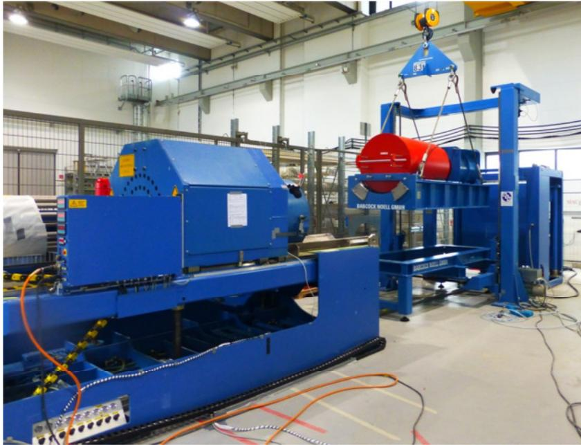
Figure 5: Mock-up for the exchange of the beamline plug JMA16 with the plug replacement machine in the neutron guide hall east.
