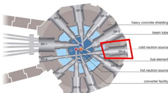
Figure 2: Section of the reactor pool with the beam tubes, the position of the beamline plug JMA16 is marked.
