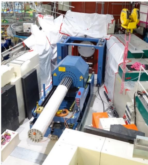
Figure 6: plug replacement machine in front of the beamline six in the experimental hall before the replacement started. The plug is still behind a closure plate.
