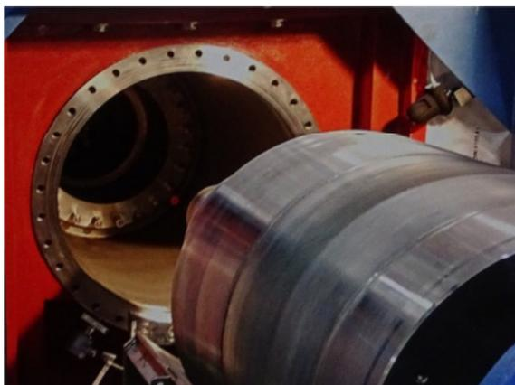
Figure 9: New plug gets pushed into the beamline.
