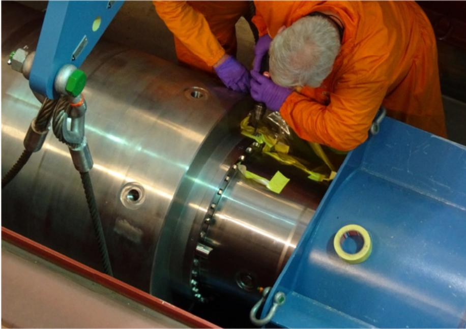
Figure 8: Drilling the samples out of the plug
