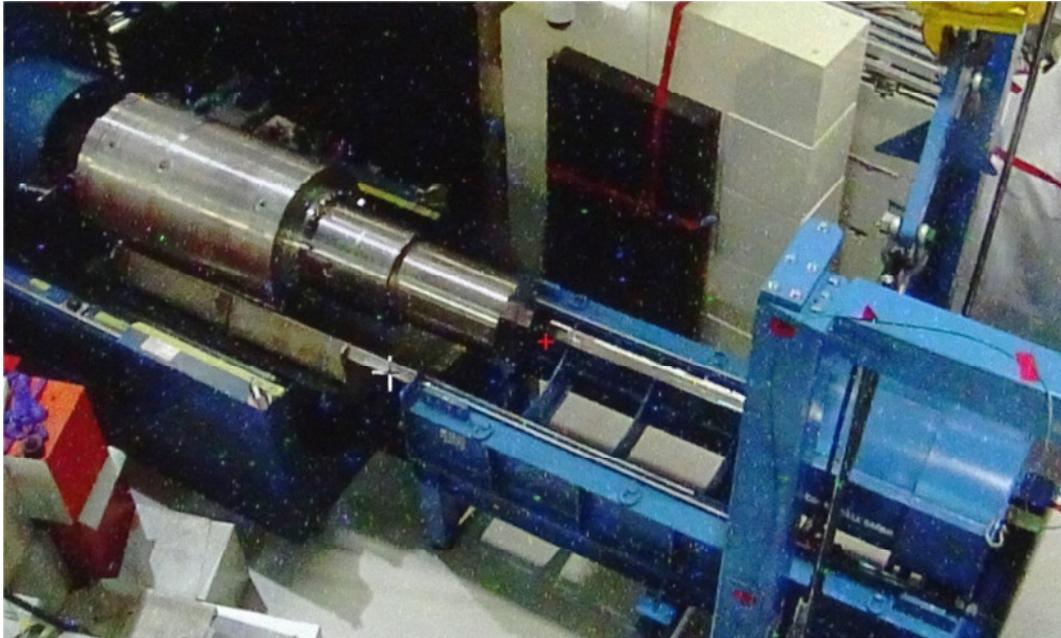
**Figure 7: The former plug already pulled out, positioned in front of the plug nose shielding**
