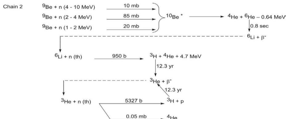
Fig. 1 (n, $\alpha$ ) triggered reaction in beryllium taken into account in calculations.
