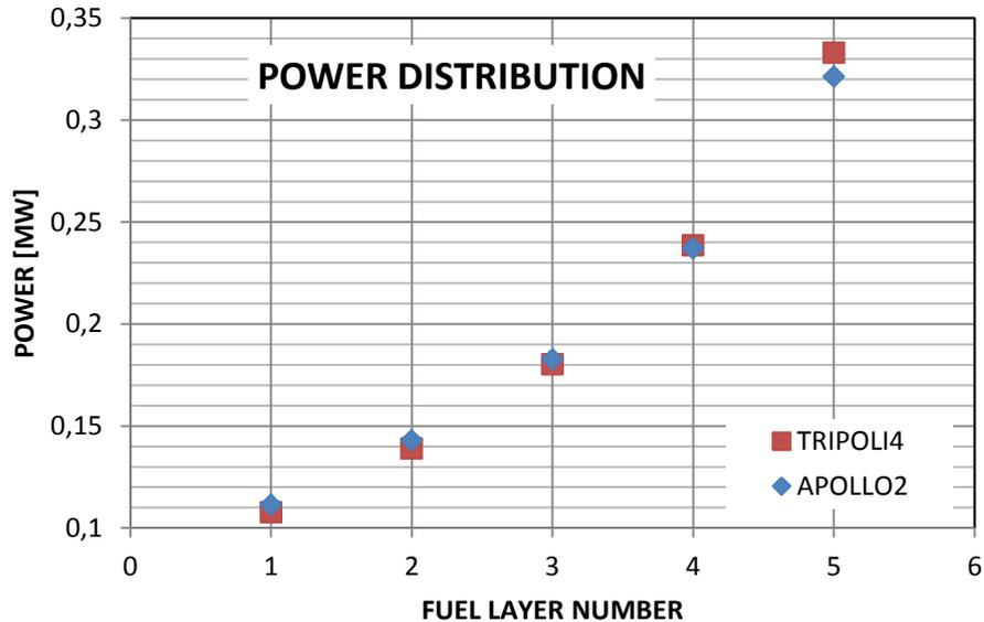
Fig. 12. Power distribution in fuel layers APOLLO2 vs TRIPOLI4.
