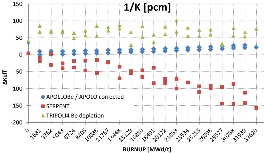
Fig. 11. Multiplication factor discrepancies – calculations with the corrected APOLLO2 depletion chain as a reference.
