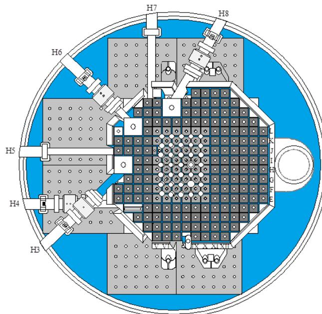
Fig. 4 Horizontal cross section of the reactor
