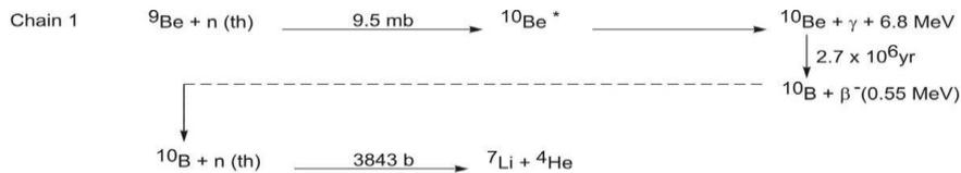
Fig. 2 (n, $\gamma$ ) triggered reaction in beryllium taken into account in calculations.
