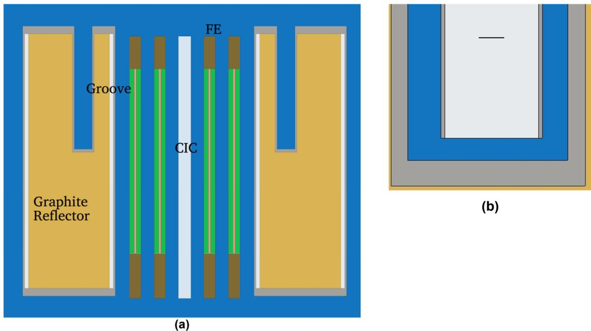
**Figure 4: (a)The vertical section of the TRIGA core modeled with Serpent-2. (b) detail of irradiated foils in the LS1 irradiation position.**
