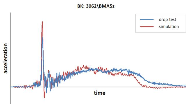
Figure 4: Accelerometer signal from slap-down drop test in comparison to FE simulation
