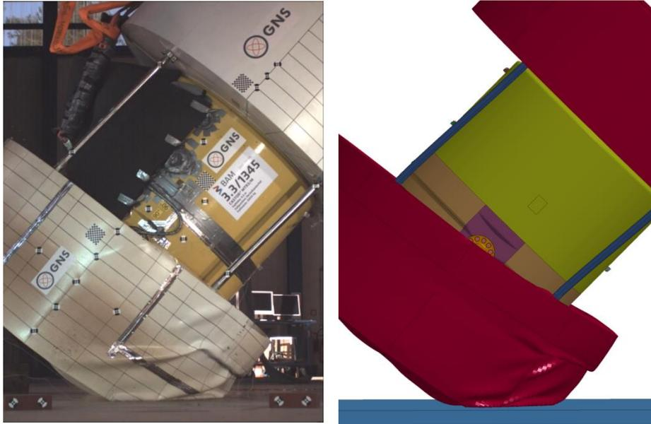
Figure 5: 9.3 meter slap-down drop test. Left: still image from high-speed video. Right: Visualisation of corresponding FE-Simulation for the same time.
