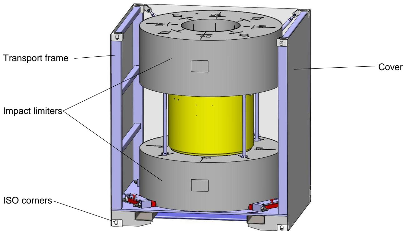
Figure 2: Transport configuration CASTOR<sup>®</sup> MTR3 with impact limiters on the transport frame (front and top side of the cover are not shown)
