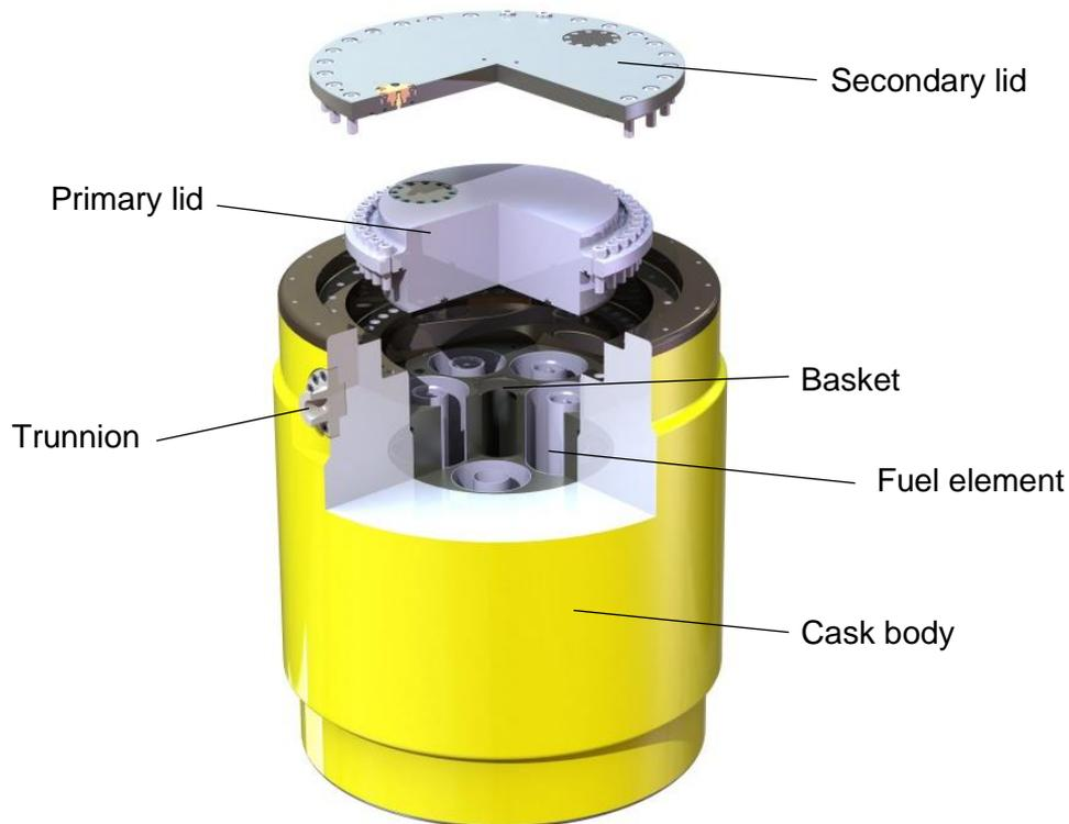
Figure 1: CASTOR<sup>®</sup> MTR3 exploded view
