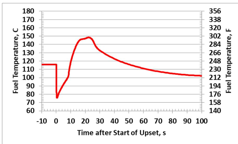
Figure 2. Peak Fuel Centerline Temperature during a Loss of Flow Accident – HEU Core
