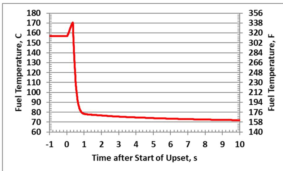
Figure 3. Peak Fuel Centerline Temperature during a Loss of Flow Accident – LEU Core
