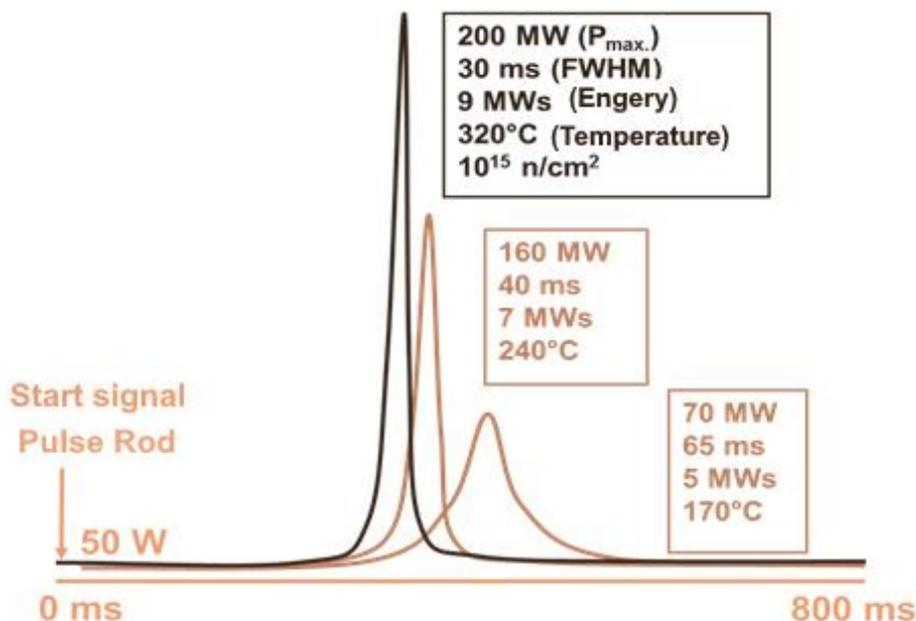
Fig. 3: Time structure of a 2 \$, 1.75 \$ and 1.5 \$ neutron pulse at the FR MZ with exemplary values for the maximum thermal power, the full width half maximum (FWHM), the pulse energy and the fuel temperature.
