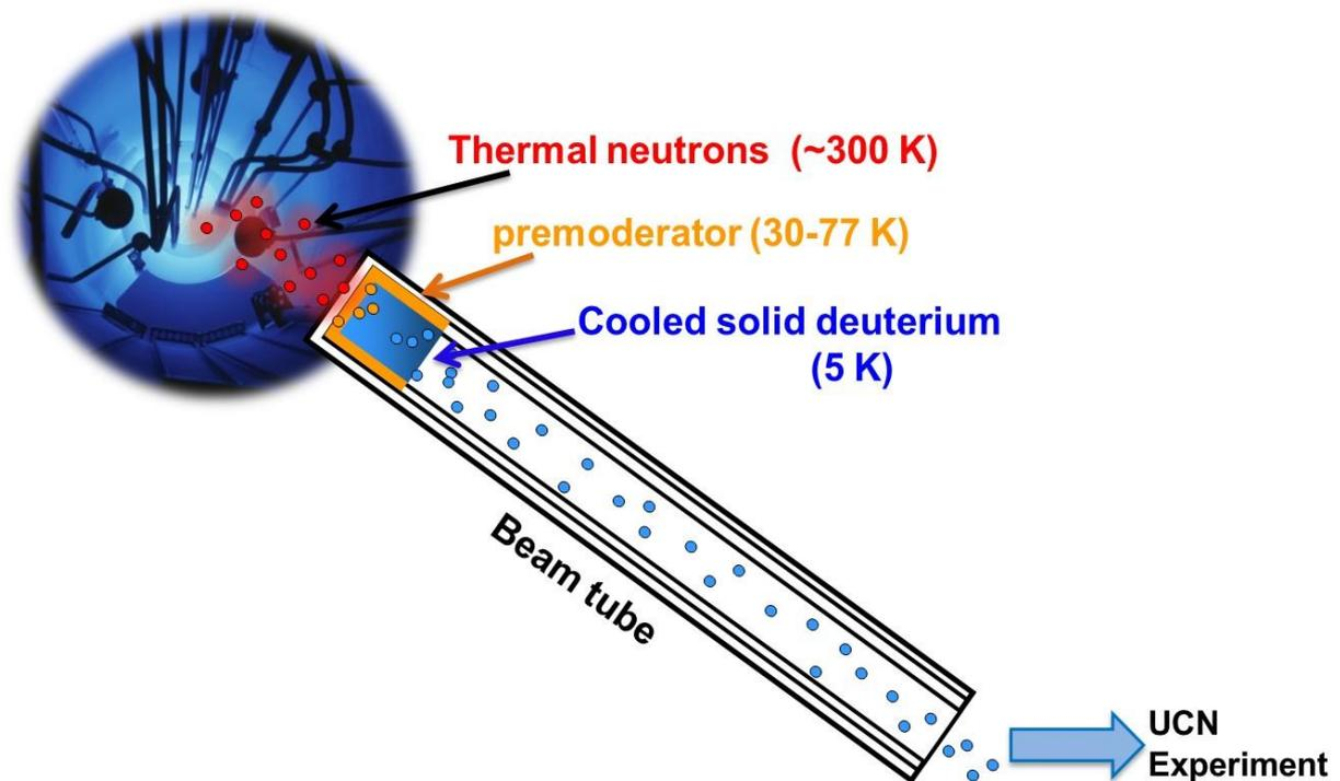
Fig. 5: Schematic presentation of the production of UCN. It shows how the thermal neutrons (red) are cooled down by a premoderator (yellow)
