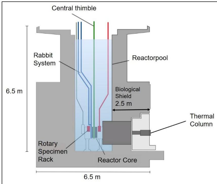
Fig. 1: Simplified drawing showing the longitudinal section of the reactor. The experimental stations are shown in this picture: in green the central thimble, in red the rotary specimen rack and in blue the pneumatically operated "rabbit" systems.
