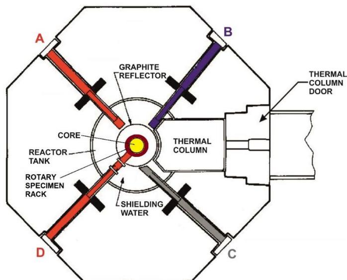
Fig. 2: Simplified cut drawing (cross section, slightly above the core center) showing the rotary specimen rack, the four beam tubes A – D, the reflector, the thermal column and the core
