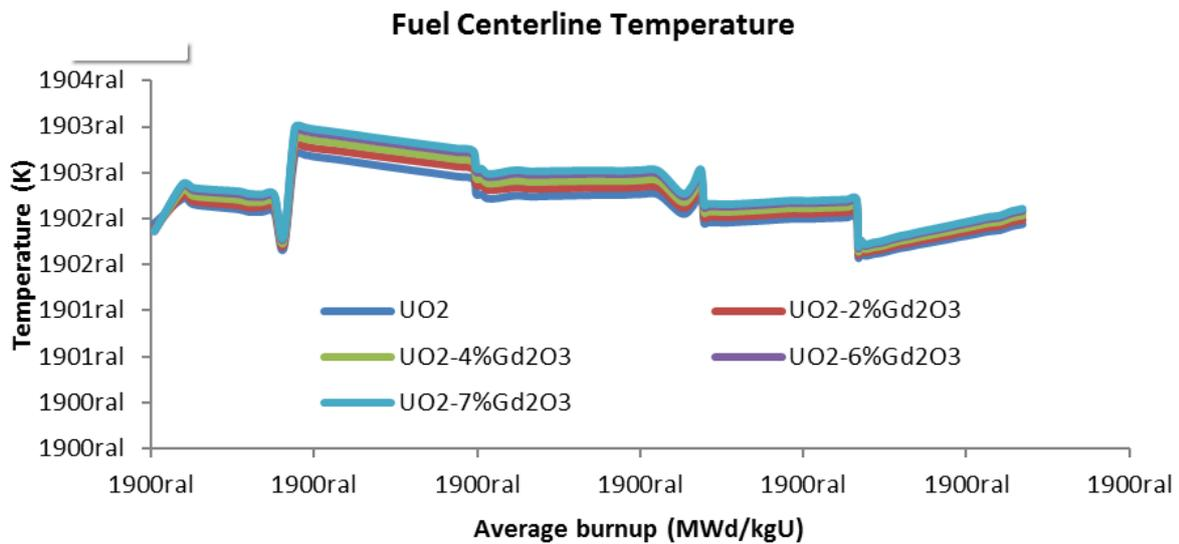
Figure 2. Fuel Centerline Temperature – UO<sub>2</sub> and the fraction of 2 a 7% of Gadolinium by weight.
