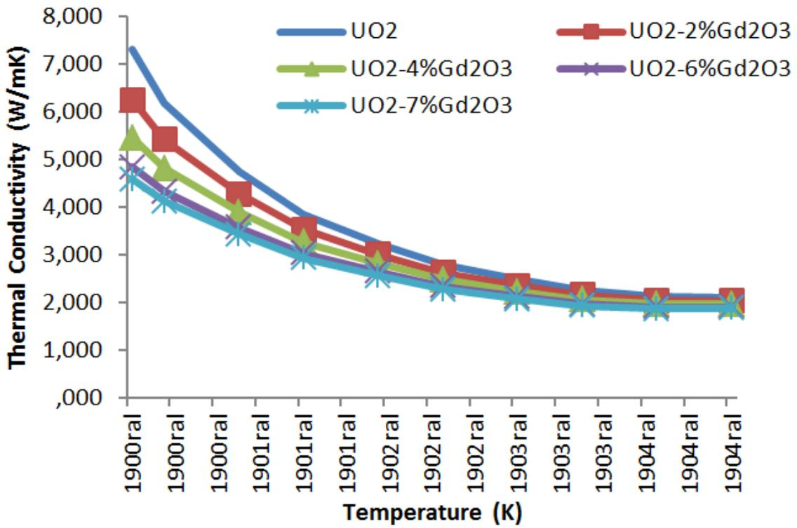
Figure 1. Thermal conductivity as a function of temperature for different concentrations of gadolinium.
