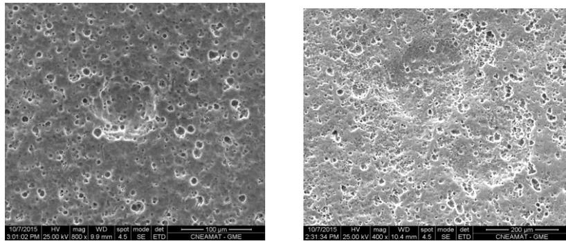
Fig 4. Example of corrosion under biofilm-oxide patches.
