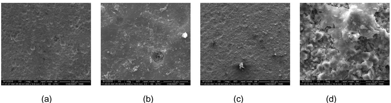
Fig 3. Biofilms on AA 6061 coupons. (a-b) Clear zones. (c-d) Black oxide covered zones.
