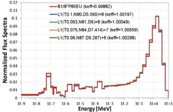
Figure 11. Central flux spectra of B1/8" P80HEU and L1 type LEU cores
