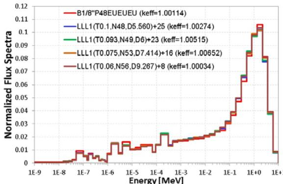
Figure 13. Central flux spectra of B1/8" P48HEU-HEU and LLL1 type LEU cores
