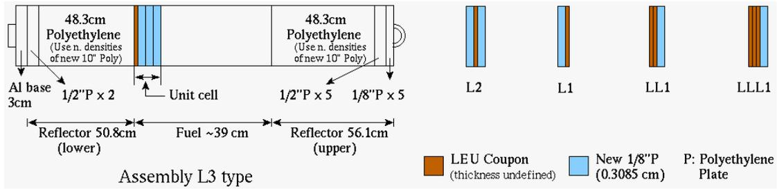
Figure 2. Axial representation of a fuel assembly model in the L3 type LEU core
