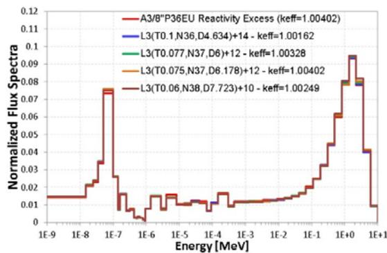
Figure 4. Central flux spectra of A3/8”P36HEU and L3 type LEU cores
