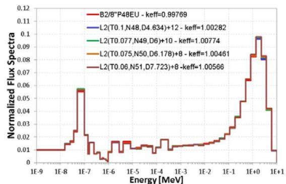
Figure 5. Central flux spectra of B2/8”P48HEU and L2 type LEU cores
