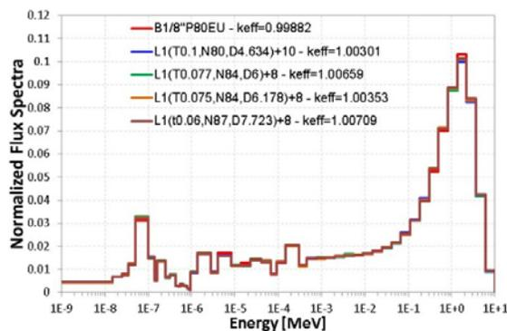
Figure 6. Central flux spectra of B1/8”P80HEU and L1 type LEU cores
