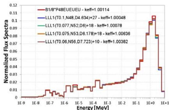
Figure 8. Central flux spectra of B1/8”P48HEU-HEU and LLL1 type LEU cores
