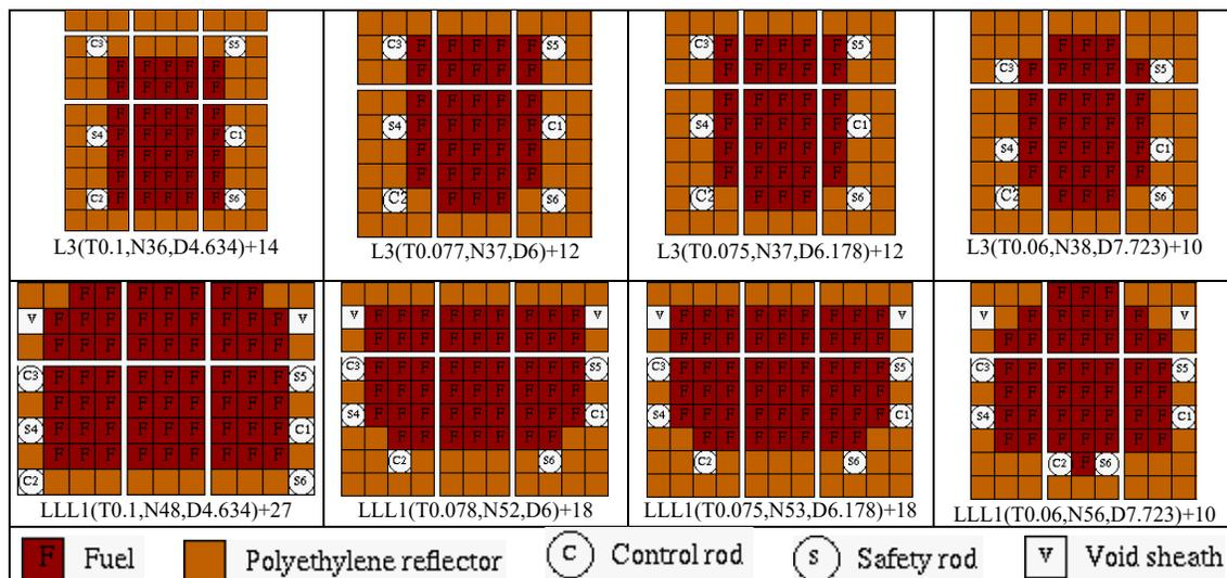
Figure 3. L3 and LLL1 type core configurations
