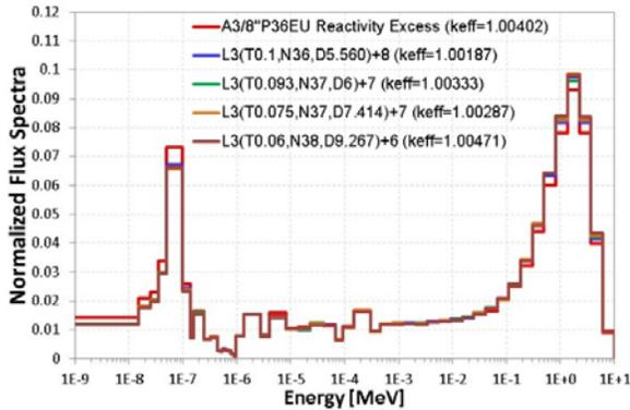
Figure 9. Central flux spectra of A3/8" P36HEU and L3 Type LEU cores
