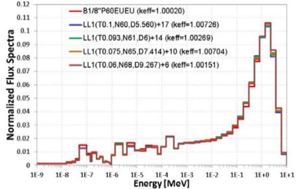
Figure 12. Central flux spectra of B1/8" P60HEU-HEU and LL1 type LEU cores
