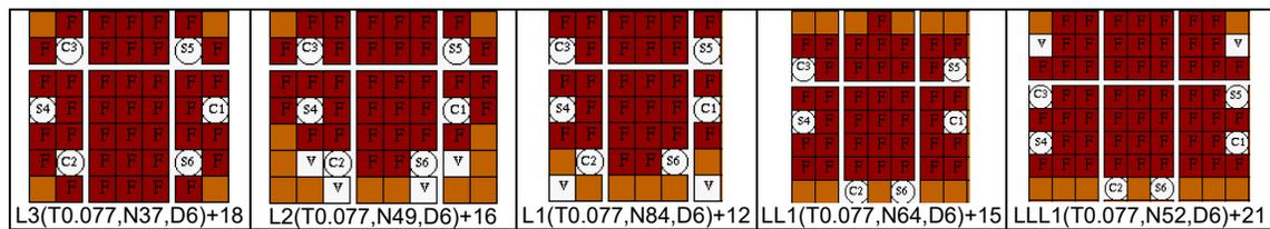
Figure 14. LEU cores configurations satisfying CR worth requirements (with coupons of 6 gU/cc and 10 g U7Mo/coupon)
