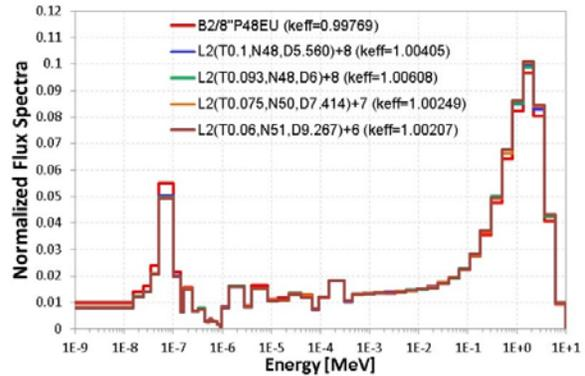
Figure 10. Central flux spectra of B2/8" P48HEU and L2 type LEU cores
