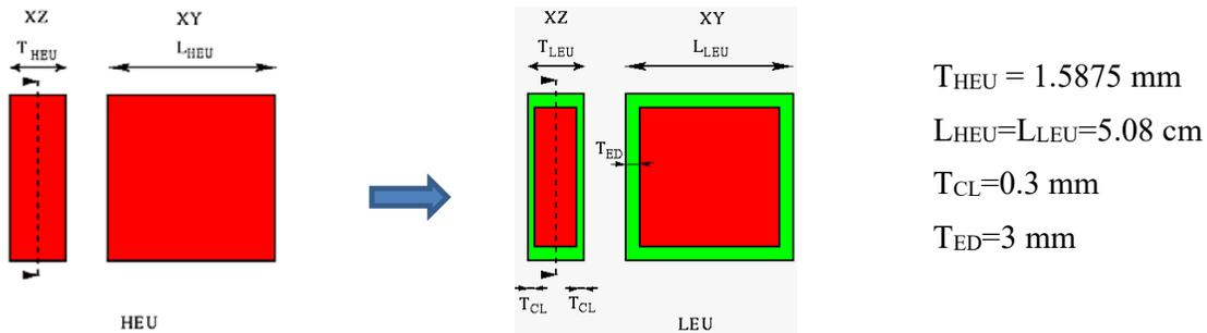
Figure 1. Configuration of HEU plate and LEU fuel coupon with aluminum edge
