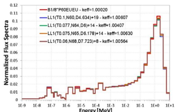
Figure 7. Central flux spectra of B1/8”P60HEU-HEU and LL1 type LEU cores
