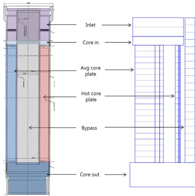
Figure 5-1: Assignment of FRM-II core geometry to ATHLET nodalisation
