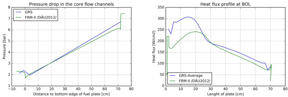
**Figure 5-2: Calculated pressure drop (left) and heat flux profile (right) compared to reference data /DÄU2012/**
