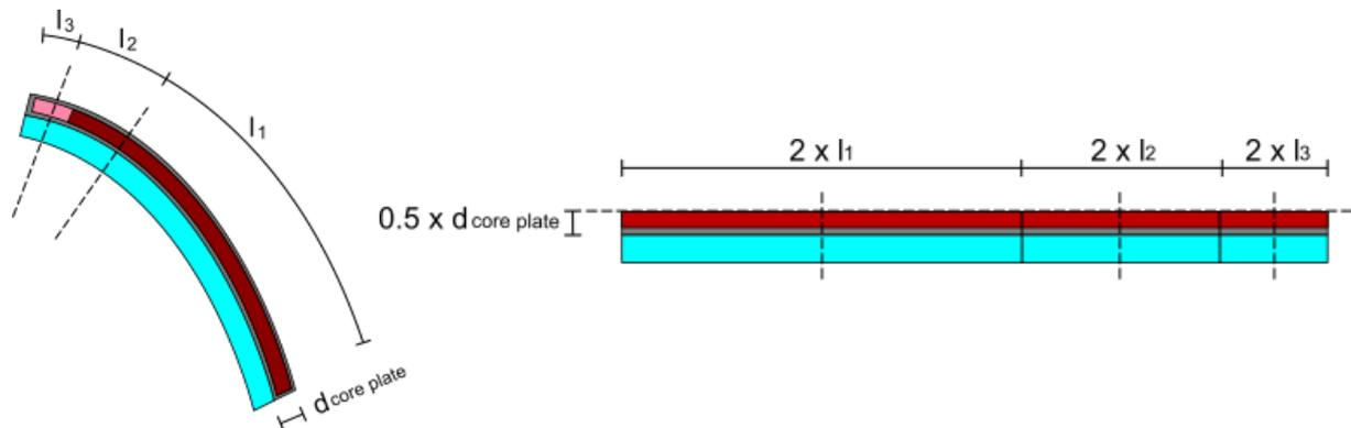
Figure 4-3: Scheme of one cooling channel subdivided into three segments (left) and model approach of corresponding heat structures in ATHLET (right)
