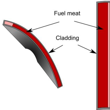
Figure 4-2: Scheme of top view (left) and front view (right) of reference fuel element; the density jump within the fuel meat is marked as light red
