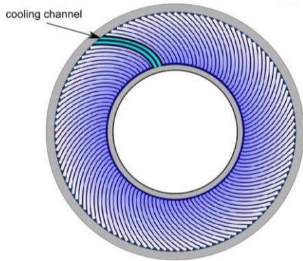
Figure 4-1: Scheme of reference compact core design; two cooling channels are emphasised in light blue
