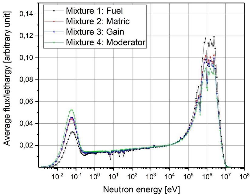
Fig. 4 Flux/lethargy vs. neutron energy in each part of the final optimized cell.
