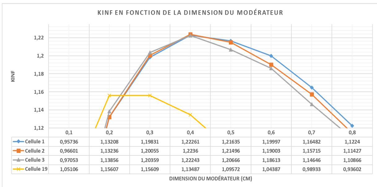
Fig. 2c : Kinf variation according to the moderator dimension in case of (Pu-Th) $O_2$  fuel with 1cm height
