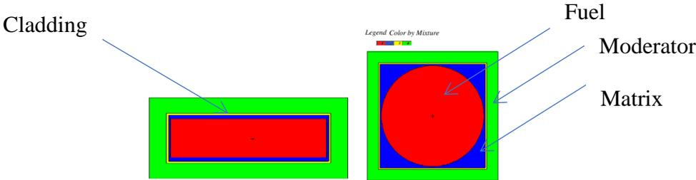
Fig. 1: Unit cuboid cell design structure; On the left: front view of unit cell; On the right: top view of unit cell
