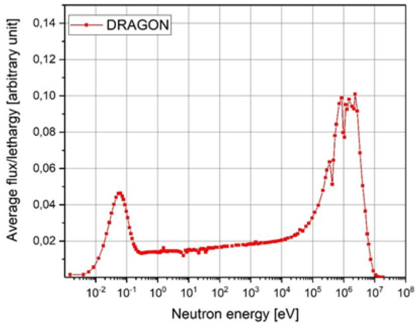
Fig. 3 Homogenized unit cell flux/lethargy vs. neutron energy calculated using DRAGON code
