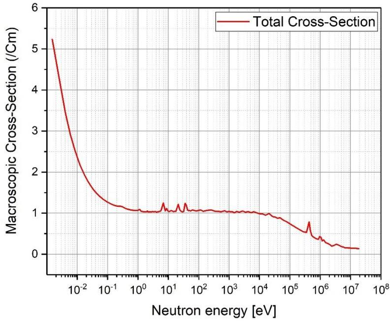
Fig.5 Total Macroscopic Cross-Section vs. Neutron energy
