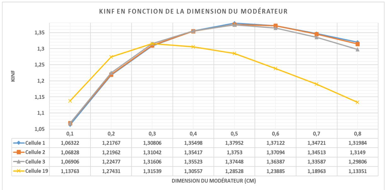
Fig. 2b : kinf variation according to the moderator dimension in case of MOX fuel with 1cm height
