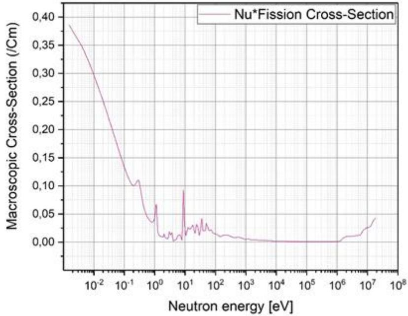
Fig. 6 Nu-Fission Macroscopic Cross-Section vs. Neutron energy
