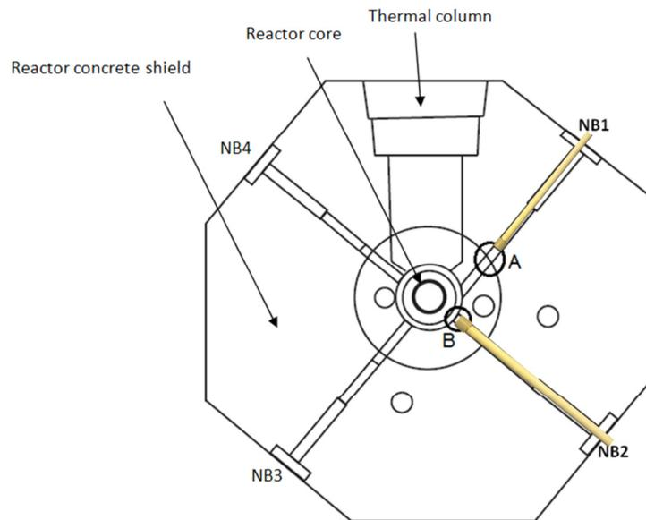
Figure 2: Top view of the TMR II reactor and irradiation positions (A position in NB1 and B position in NB2)
