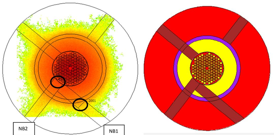
Figure 3: MCNP model for TMR II with calculation positions and particle source distribution
