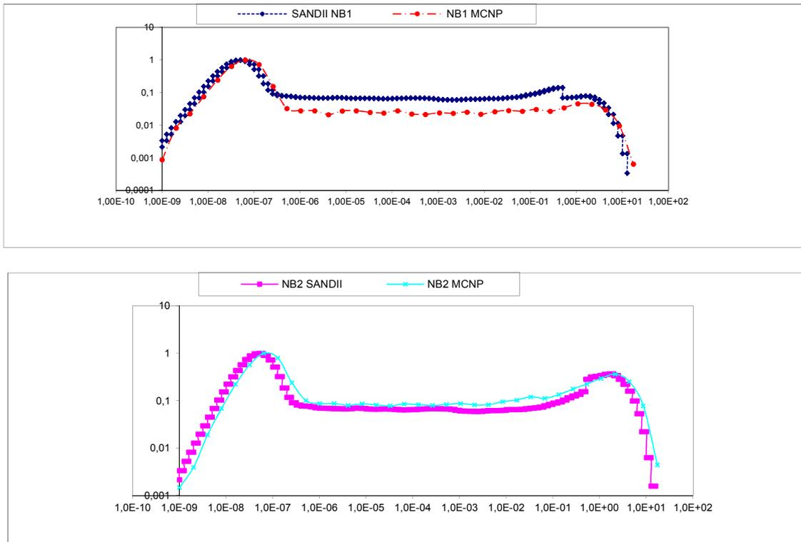
Figure 4: Spectra comparison for NB1 and NB2 determined by SAND II and MCNPX
