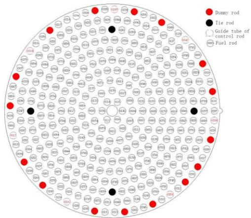
Fig. 5 The arrangement of the fuel elements.
