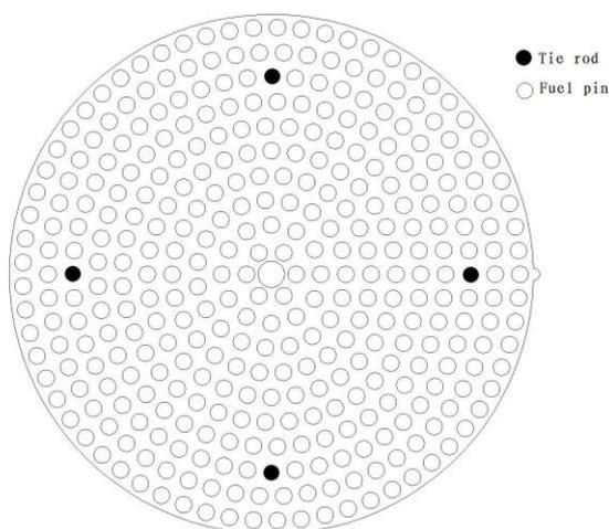
Fig. 2 The diagram of fuel arrangement
