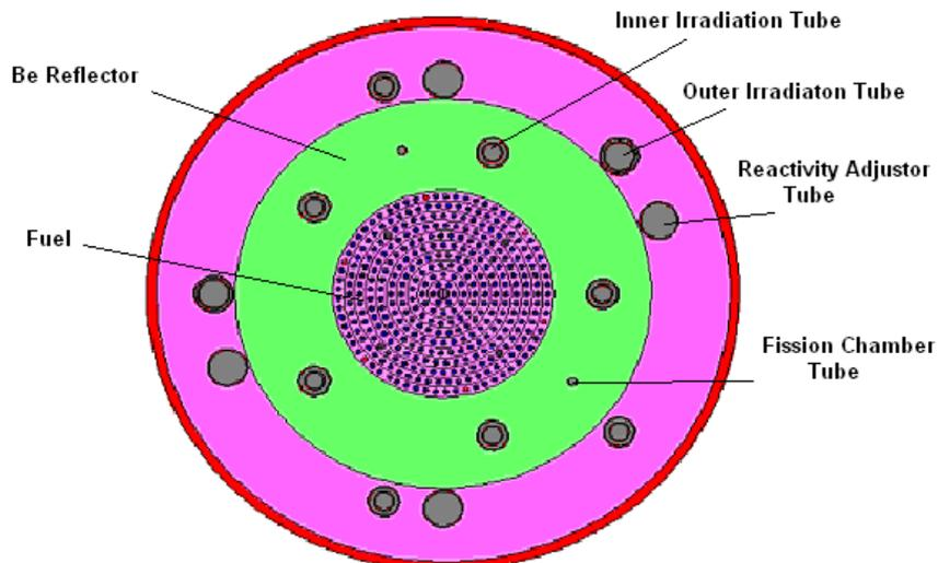
Fig.1 The diagram of the experimental equipment
