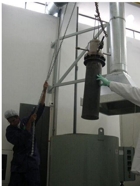
Figure 1. Charging of the reactor vessel inside the pit furnace
