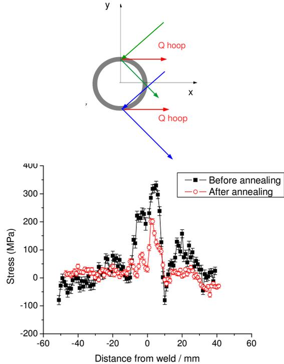
Fig. 7. Radial stresses in the vicinity of the test weld
