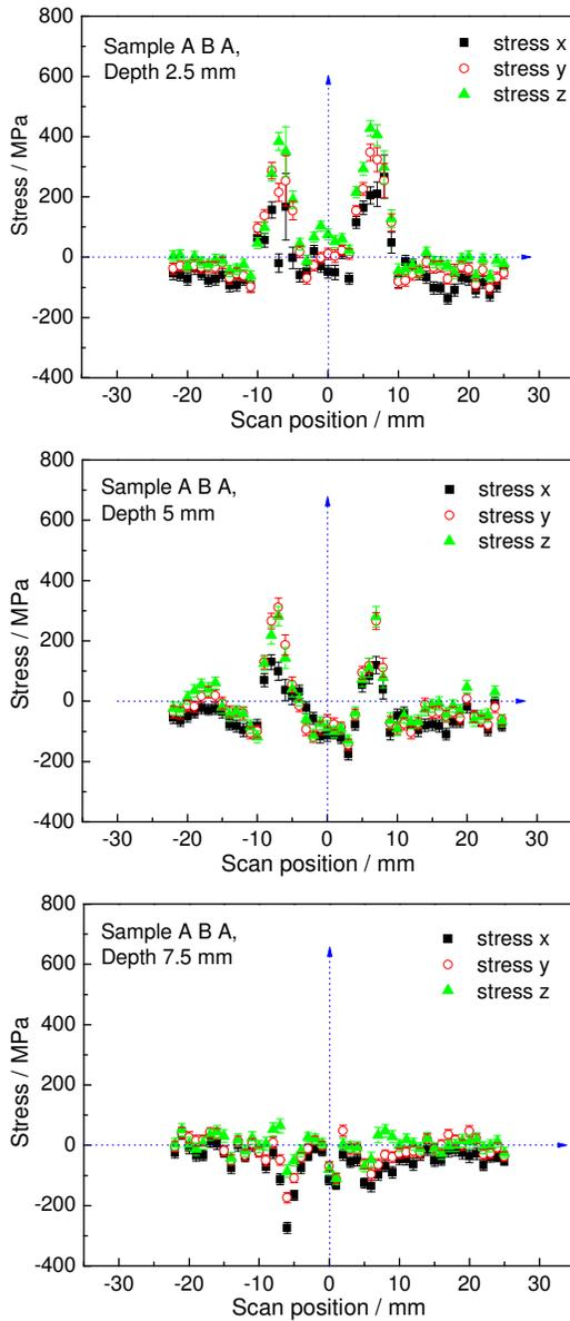
Fig. 10. Residual stress scans performed at different depths in the material for the sample with the weld on both sides
