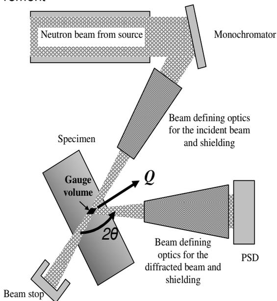
Fig. 2. Sketch of the sample setting for determination of three strain/stress components
