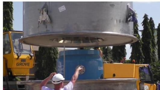
Fig. 2. The ŠKODA VPVR/M cask inside the TUK-145/C Energy Absorbing Container
