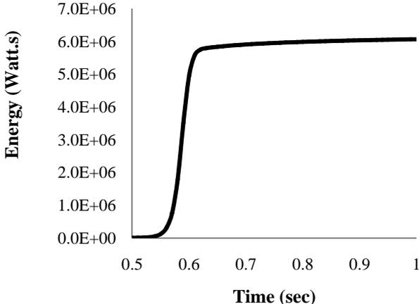
Fig. 3: Time behaviour of energy release in fast reactivity insertion (1.4 \$ per 0.5 sec)
