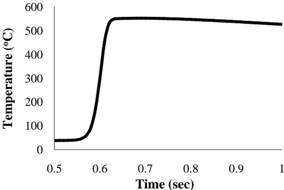
Fig. 4: Time behaviour of clad temperature in fast reactivity insertion (1.4 \$ per 0.5 sec)
