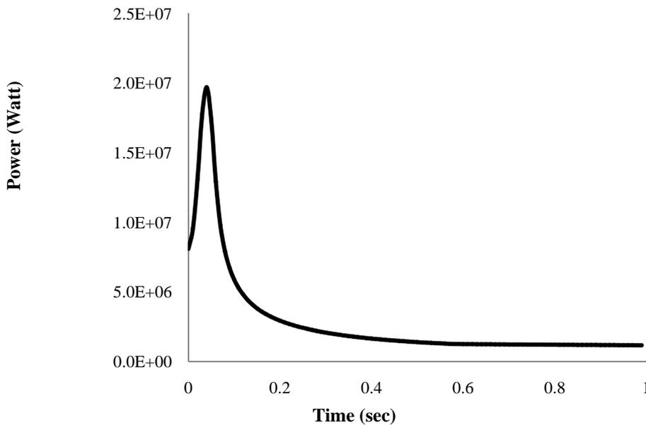
Fig. 5: Time behaviour of power for removal of in-pile experiment
