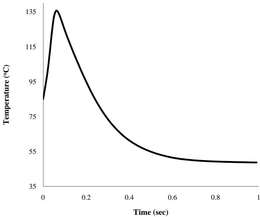
Fig. 7: Time behaviour of clad temperature in removal of in-pile experiment
