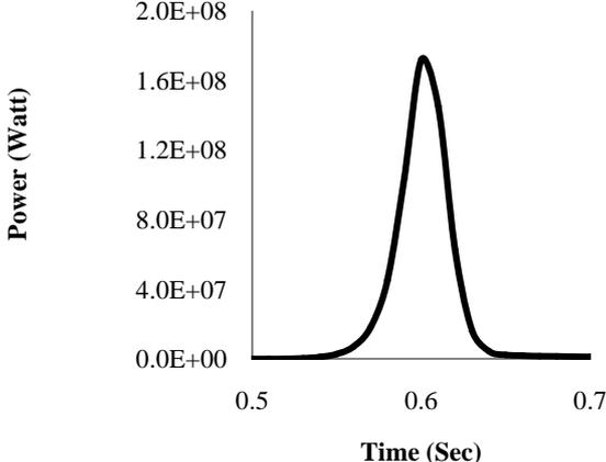
Fig. 2: Time behaviour of in fast reactivity insertion (1.4 \$ per 0.5 sec)
