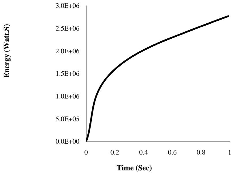
Fig. 6: Time behaviour of energy released in removal of in-pile experiment
