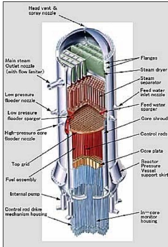
Traditional Advanced Boiling Water Reactor (Hitachi-ABWR)
