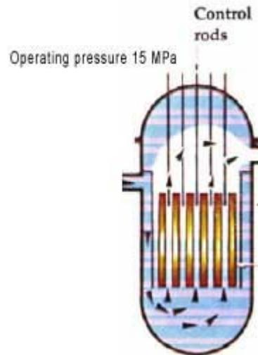
The control rods are operated from above. Undoubtedly some leakages were observed at the penetrations which in a few cases led to the need to replace the reactor pressure vessel head.
