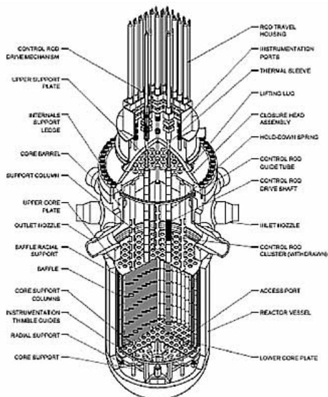
The simple electromagnetic devices which manoeuvre the rods worked reliably. This assures a high degree of safety. A basically continuous, uninterrupted bottom of the reactor vessel avoids any suspicions of its integrity.
