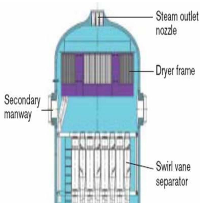
In the upper part of the steam generators there is the moisture separator and the steam dryer. The HP-BWR is “borrowing” this equipment which can be used without the troublesome steam generators.
