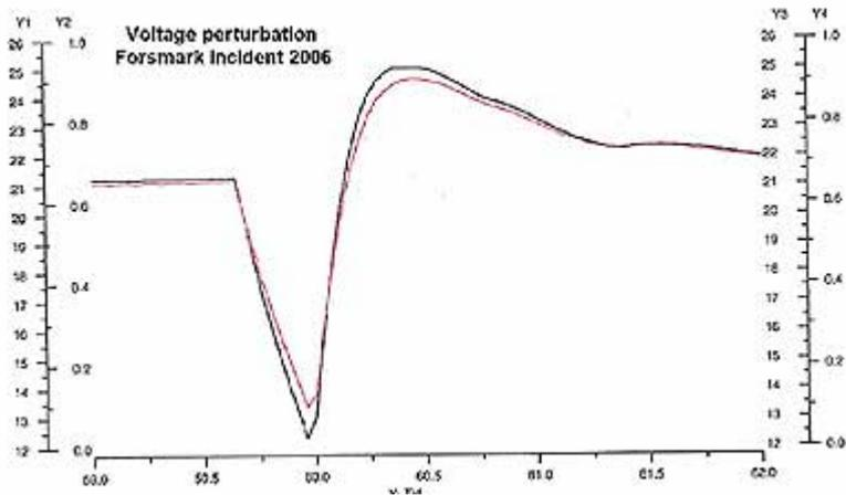
The main generator's low frequency protection was installed with erroneous phase order and therefore did not disconnect the 20 kV generator breakers in time. That disconnection would have connected in an alternative (70 kV) power supply. The alternative power supply, like the diesels were connected in to the system manually some twenty minutes later.
